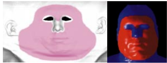
Figure 7: Setting of the boundary conditions by defining a texture map. Left: Texture map, right: Visualized boundary conditions.
