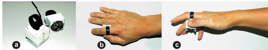
Fig. 8. (a) The cubeRing design with an adjustable finger ring on the top, and a small cube on the bottom. The cubeRing can be worn in the index finger, and operated on the desktop surface (b) and in hand-held position (c).
