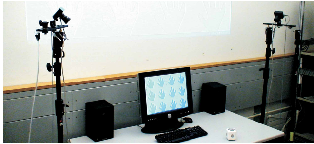
Fig. 3. A prototype setup with a pair of video cameras, the mCube device, a desktop monitor, and a large display wall for wall projections.
