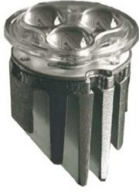
Figure 3.10: LED light unit - A light unit is equipped with red, green and blue LEDs (Philips Lumileds LUXEON K2) as well as a 45° lens and a heat sink. The table lists specifications for the used LEDs. The unit consumes approximately 8 Watts at full operation and produces 200-240 Lumen.
