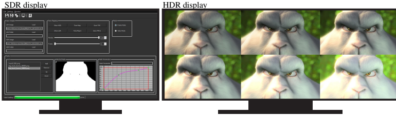
Figure 6.3: This figure shows our luminance grading interface. On the SDR display, masks with values in [0, 1] can be loaded in the bottom left menu, and are displayed in the bottom-middle window. A cubic spline interface shown on the bottom right allows the user to manually input lumipaths. Different visualization options can be selected from the menu on the top. On the HDR display, users can visualize their edits in an interactive manner. To see a standard work session using our interface, we point the reader to the supplementary material of the corresponding publication [Chapiro et al., 2015a]
