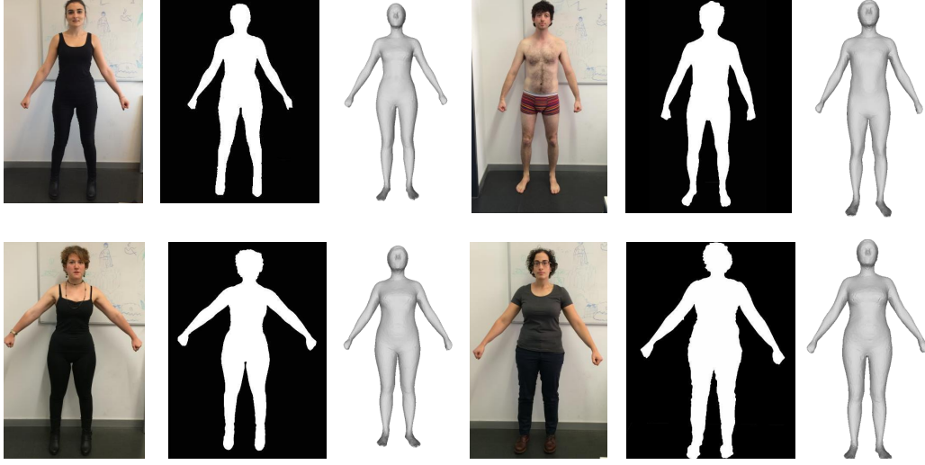
Figure 3.15: Mesh reconstruction for 4 real subjects in mildly varying poses. (left) Input image (middle) Extracted Silhouette (right) Reconstruction of the estimated shape.
