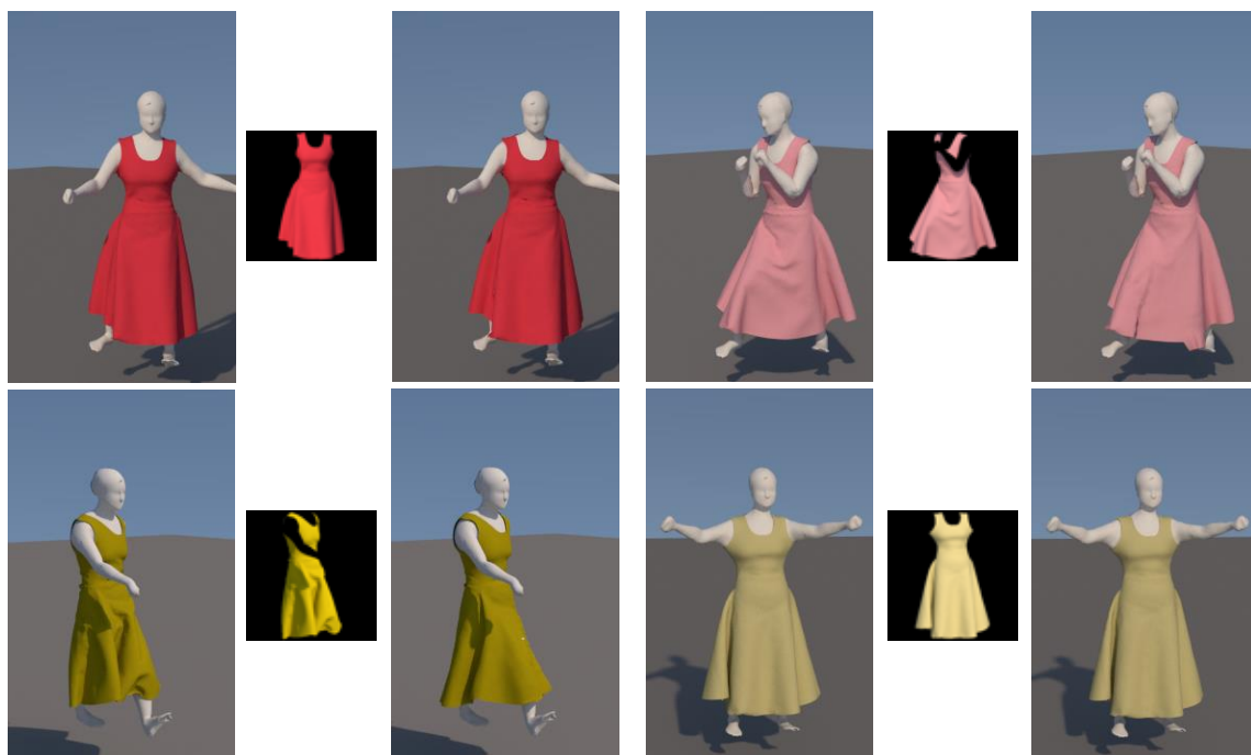
Figure 4.8: Recovered garment shapes with the "Garment-from-Body" representation. From left to right: initial rendering, segmented dress and rendering of the same scene using the estimated mesh.
