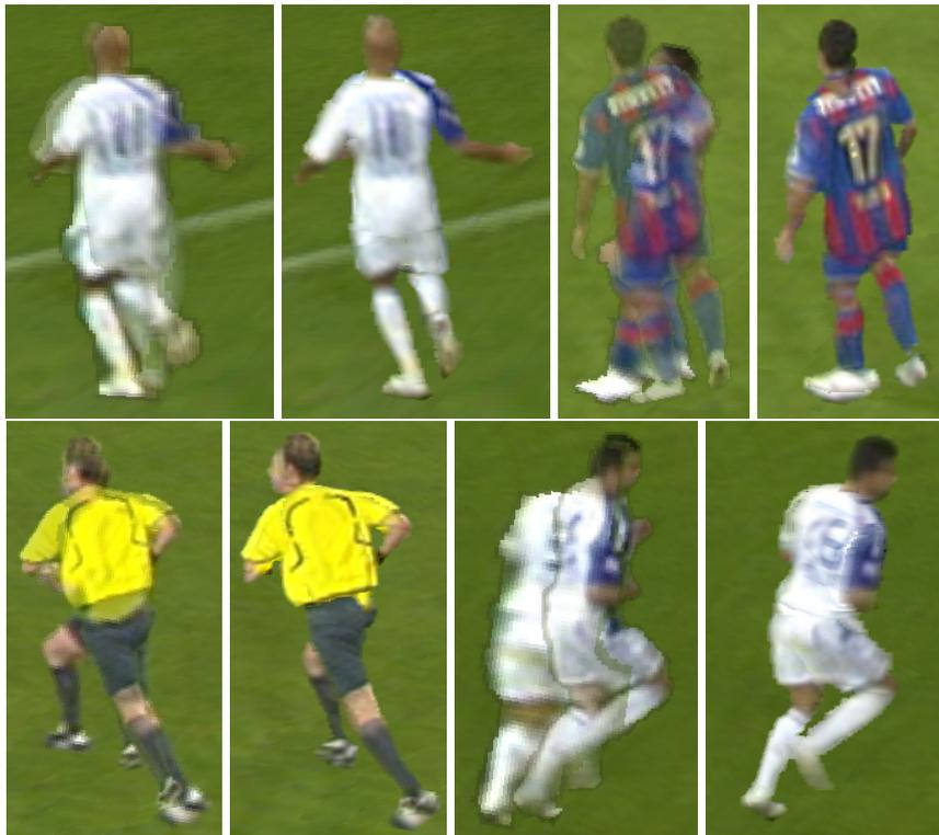
**Figure 6.9:** Direct comparison for views in the middle of two source cameras. Each player is rendered with a standard billboard technique and with articulated billboards. The standard billboards exhibit considerable ghosting artifacts.
