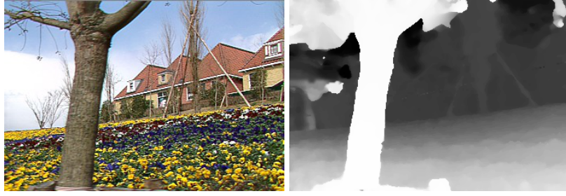
Figure 4.12: Result on the Flower Garden sequence with 50 images. Left: One input image with 0.08 MP resolution. Right: Our depth map. The computation time was 3 seconds.
