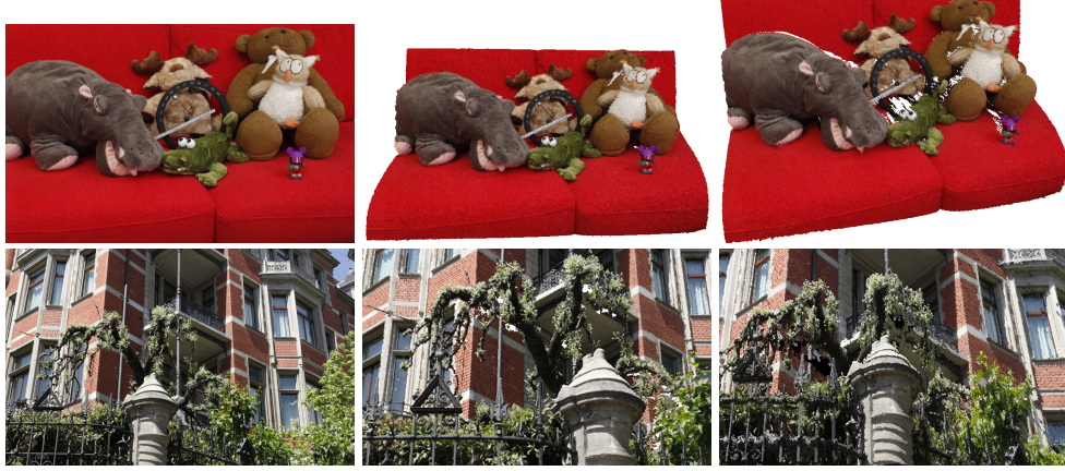
Figure 4.16: Examples for novel view-synthesis by rendering a colored point cloud. The leftmost image is from the set of input images.
