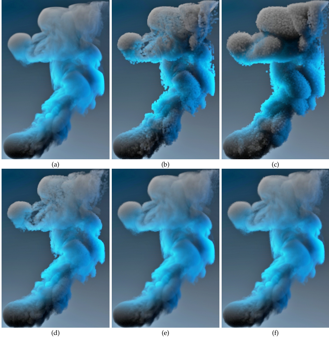
Figure 5.7: Comparison of different re-simulation strategies. (a): ground truth density, (b): constant density carried by particles, (c): (b) with redistribution by Equation (5.6), (d): single-scale sampled density, (e): (d) with redistribution, (f): multi-scale ( n_s = 3 ) sampled density with redistribution (final method).
