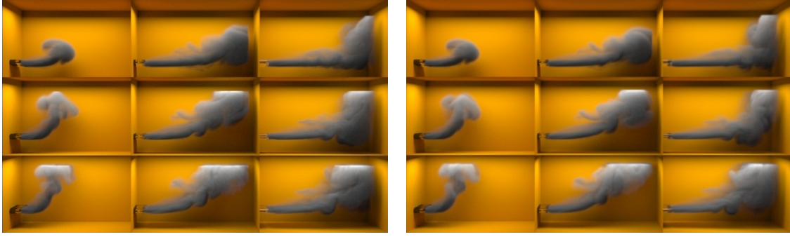
Figure 3.2: Ground truth (left) and the CNN-reconstructed results (right) for nine sample simulations with varying buoyancy (rows) and inflow velocity (columns). Despite the varying dynamics of the ground truth simulations, our trained model closely reconstructs the reference data.
