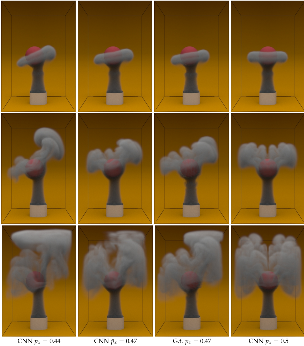
Figure 3.12: Interpolated result (second column) given two input simulations (left and right) with different obstacle positions on the x -axis. Our method results in plausible in-betweens compared to ground truth (third column) even for large differences in the input.
