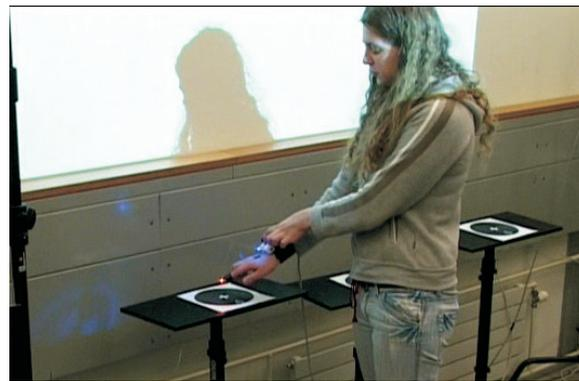
**Figure 6.3:** Registering an object using touching. A user is locating a gesture input device (mWire) at the location of the object and registering the positional data to the system by pressing the button of the device.
