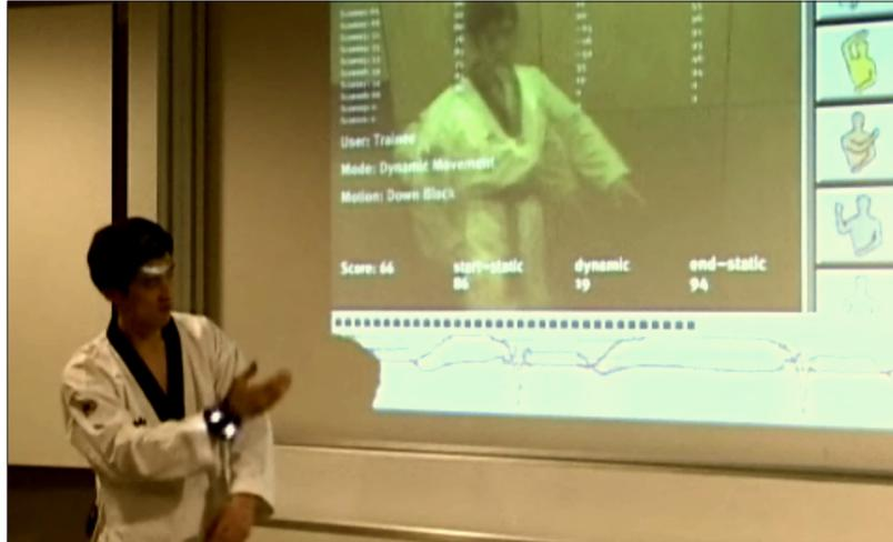
**Figure 5.8:** Gesture instruction system in action. The trainee wears body sensors on the wrist and performs a gesture watching the visual feedback on the wall display.
