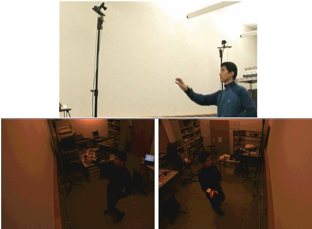
**Figure 3.7:** The prototype camera installation and views from the cameras. (Top) A user is performing a 3D spatial gesture in the prototype system setup that consists of a pair of cameras and a projection wall in front of the user. The camera is pointing down to the user. (Bottom) The images from the cameras.
