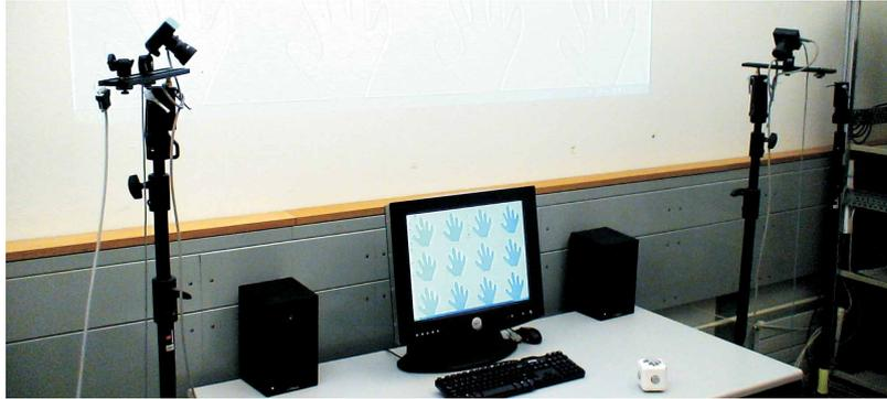
**Figure 7.2:** A prototype setup with a pair of video cameras, the mCube device, a computer with active Bluetooth wireless network, a desktop monitor, and a large display wall for wall projections.
