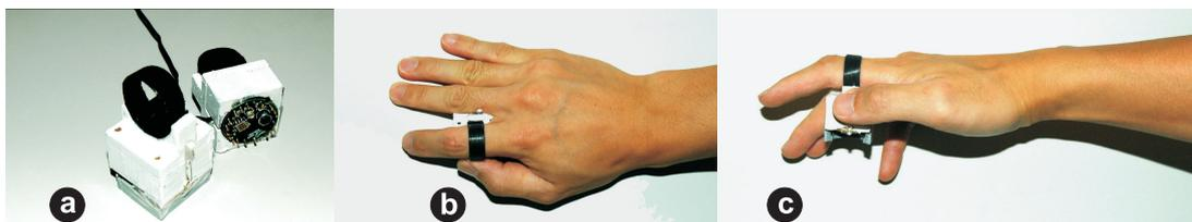
**Figure 8.3:** An example of an alternative input device design called *cubeRing*. (a) The *cubeRing* with an adjustable finger ring on the top, and a small cube on the bottom. The *cubeRing* can be worn on the index finger, and operated on a desktop surface (b) and the *cubeRing* in the hand-held position (c).
