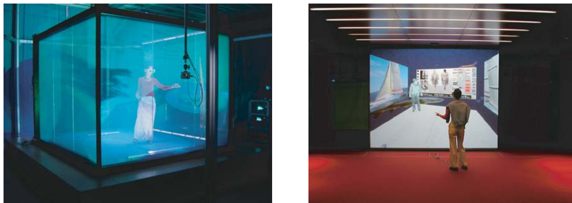
Figure 2.1: The two blue-c portals in action. The left-hand side shows a three-sided CAVE TM -like blue-c portal with three actively shuttered projection walls. The right-hand side shows a PowerWall-like blue-c portal with one projection wall. Both systems acquire the 3D video inlay with 16 cameras and have stereo projection capabilities.
