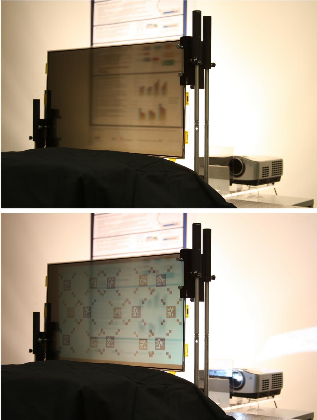
**Figure 6.4:** *Our transparent stereoscopic display prototype once without displaying anything to illustrate transparency (top) and once showing the calibration pattern that was used in our calibration algorithms (bottom). A RGB liquid crystal display is used as barrier layer losing much transparency in the embedded color filters. Using a gray-scale liquid crystal display as deployed in e.g. medical screens would improve transparency significantly.*
