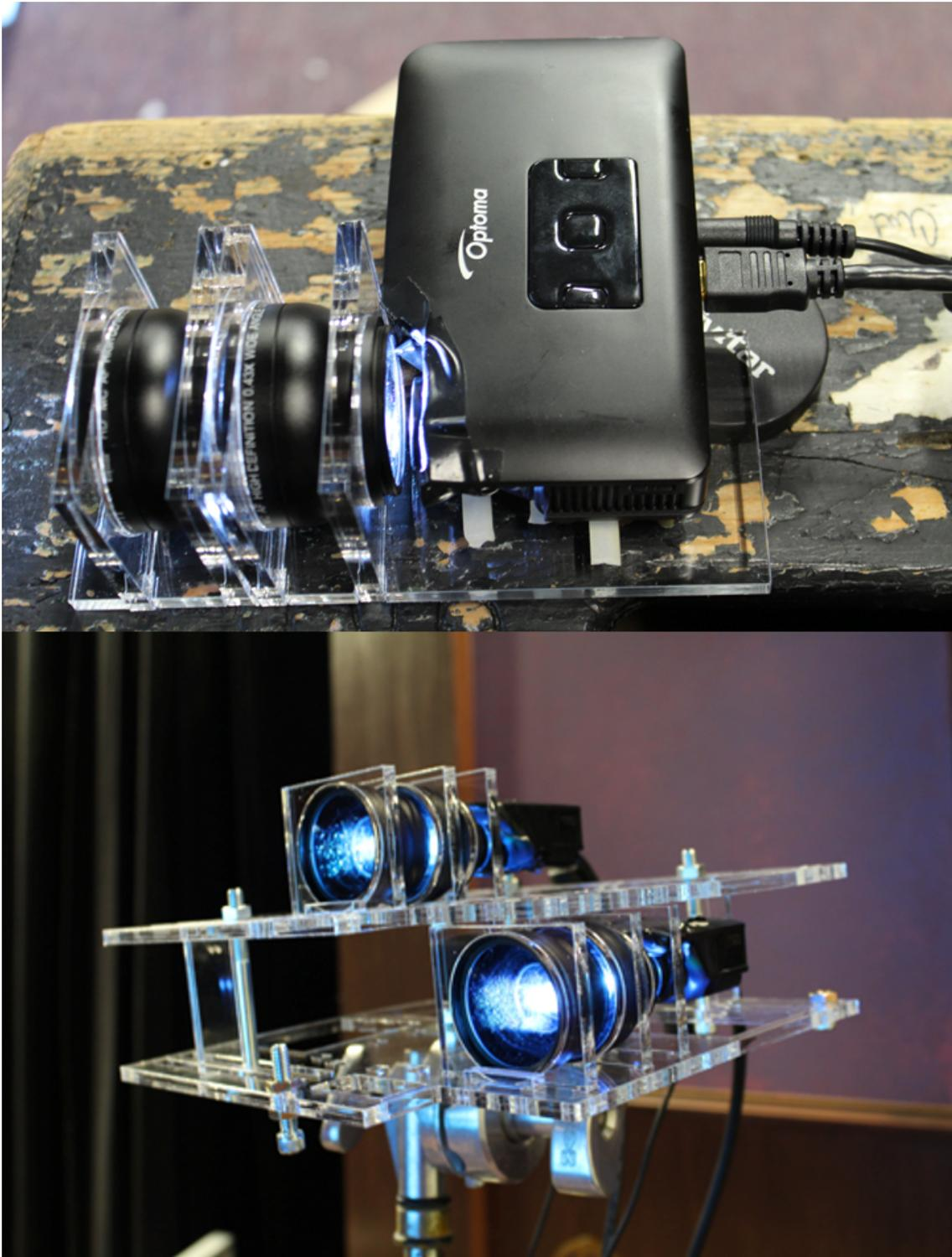
**Figure 3.7:** *Illustration of the modified Optoma microprojectors. Two concatenated wide angle lenses greatly enhance the field of view. The top image shows a single projector while the bottom image shows a stereo projector configuration.*
