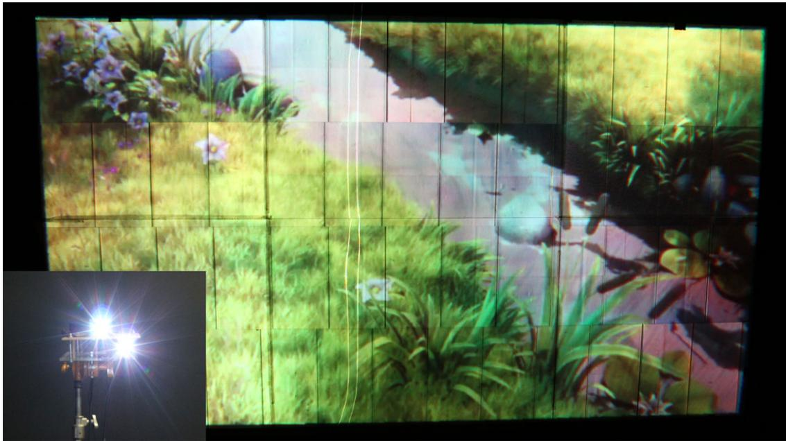
**Figure 3.11:** *The left eye image of a single stereo projector pair. Two projectors are arranged side by side with a spacing matching the average human eye distance. The image is bright due to the retroreflection and shows only very low crosstalk from the right eye image.*
