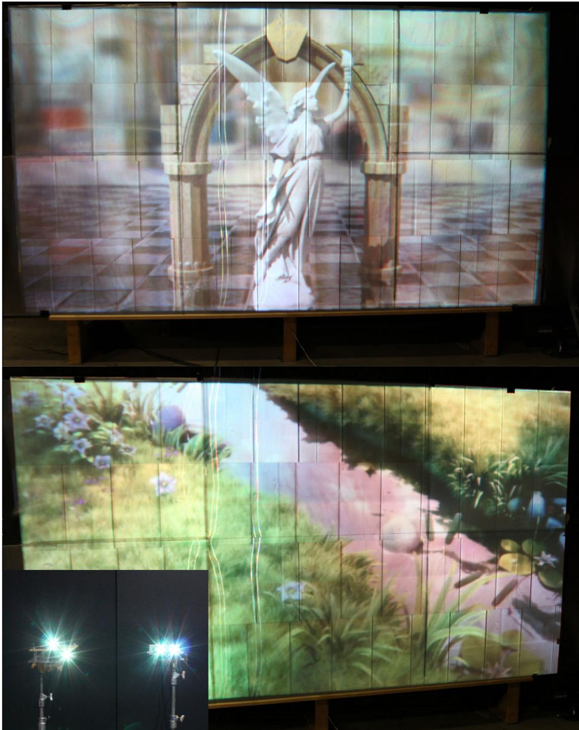
**Figure 3.14:** A stereo setup for two viewers. Two projector pairs are placed side by side. Two different stereo image pairs are exposed to each viewer. The left images of both viewers are shown in the top and in the bottom image.
