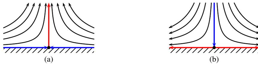
**Figure 2.16:** 2D flow separation (a) and attachment (b) represent half saddles in terms of 2D vector field topology (Figure 2.9 (c)). The critical points represent separation (a) and attachment (b) points and the separatrices the respective manifolds. For this illustration, we assume slip boundaries (hatched) or wall shear stress thereon.
