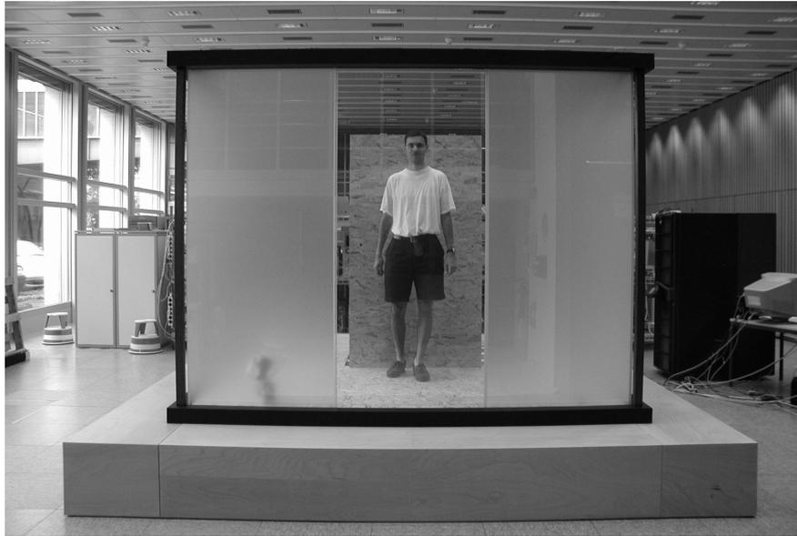
**Figure 4.1** Three PDLC glass panels, middle panel switched transparent
