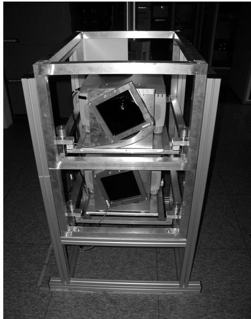
**Figure 3.6** Active LCD stereo projection system
