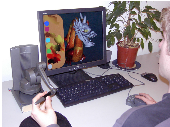
Figure 5.1: A photograph of the virtual painting system. The haptic device (left) is used to control the brush, another 6D input device (right) moves and rotates the object. Similar to the real painting process, a palette is used to mix paint.
