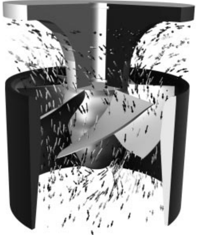
Figure 1: Simulation model of a Kaplan turbine runner, a type of water turbine often used in river power plants. This case study describes issues of visualizing results of CFD simulations for the design of such water turbines.
