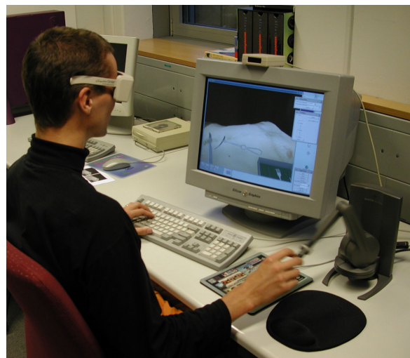
Figure 11: Simulation setup with PHANTOM ® force feedback device and stereo glasses
