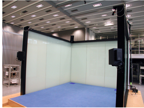
Figure 8: Setup of the blue-c with six speakers.
