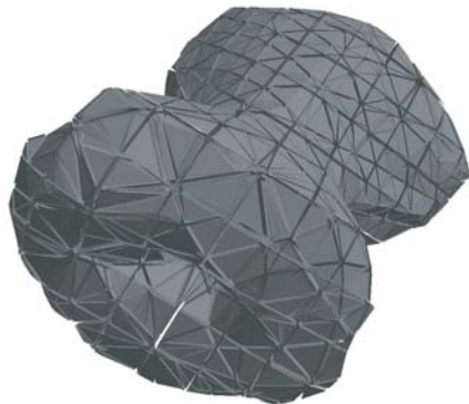
Fig. 3. In this case, the initial tetrahedral mesh (see Fig. 2) is subdivided along the triangle-based surface mesh. If a surface triangle intersects with an edge of the tetrahedral mesh, the edge is subdivided. New tetrahedrons are generated accordingly. The resulting mesh consists of 7400 tetrahedra.
