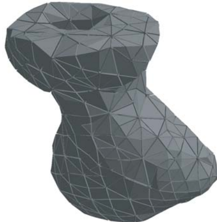
Fig. 4. Optimized mesh. Positions of all vertices (see Fig. 3) are optimized with respect to aspect ratios for all tetrahedra. Further, all boundary points of the tetrahedral mesh are constrained to lie on the initial surface mesh. In addition, tetrahedra with insufficient quality are deleted. The final mesh consists of 2400 tetrahedra.
