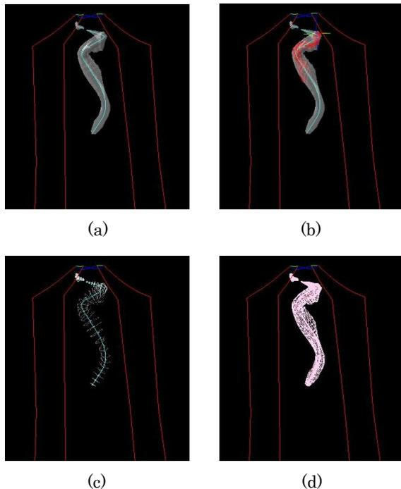
Fig. 3 A typical vortex in the turbine draft double-tube to explain each result of the vortex hull finding steps. (a) A set of last points. (b) Triangulation of the vortex. (c) Smooth vortex hull. (d) Vortex hull with manually-specified streamlines.
