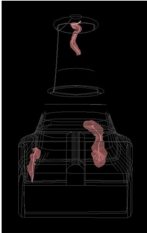
Fig. 2 Computed vortex core lines and their vortex hulls in the turbine draft double-tube.
