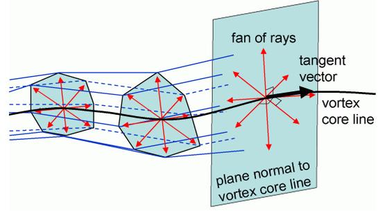
Fig. 1 Principle of the core-line-based vortex hull finding method.
