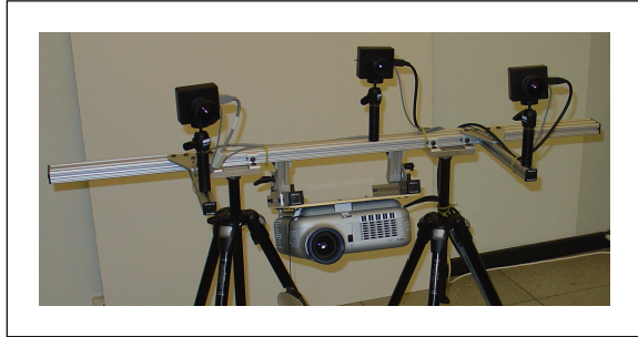
Figure 2: Instant display brick with projector and cameras.
