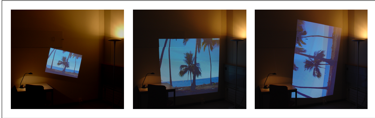
Figure 19: Interaction with instant displays projected using three bricks. Screens can be moved, scaled, rotated and changed in aspect-ratio at any time by the user with intuitive laser-pointer commands.
