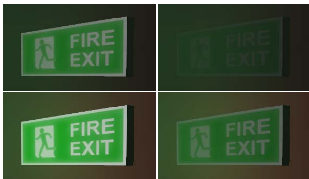
Figure 8: Illuminated exit signs (left column) are visible further than reflective exit signs (right column), which is achieved by adjustment of the transfer function.
