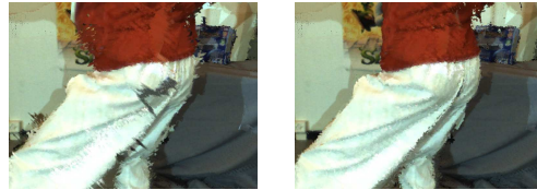
Fig. 7 Enforcing photo consistency during view merging: Without (left) and with (right) enforcement.
