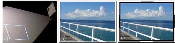
**Figure 2:** Tracking border. a) Pocket light unit projecting a white tracking border. b) Sample image with surrounding tracking frame of type A. c) Sample image with surrounding tracking frame of type B, which also encodes the orientation.
