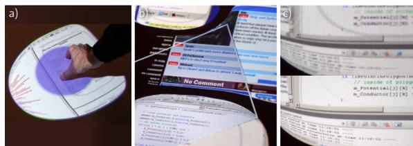
**Figure 22:** The context areas of the adaptive displays can be explored with single-handed scrolling (a) or using high-resolution foveal areas (b), selectively enhancing the legibility (c).
