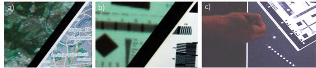
**Figure 17:** Hybrid foveal displays. a) Customized foveal area using a laptop screen. b) Resolution comparison between the LCD panel and the surrounding large-scale projection. c) The user can directly work on the ordinary screen using a light-emitting pen.
