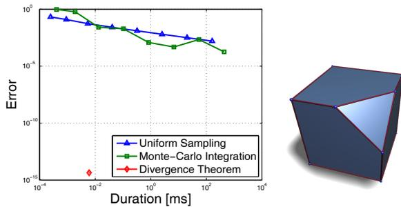
Fig. 4. Comparison of different numerical integration methods to our analytic method based on the divergence theorem. In this example the function  $f(x, y, z) = x^2$  was integrated over the corner-cut cube model shown on the right.
