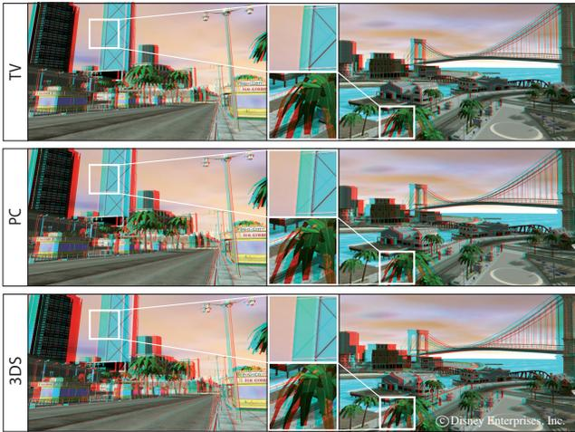
**Figure 7:** Content produced for different screen sizes. The viewing conditions and target depth ranges for each device can be found in Table 1. In the middle of each row, magnifications of certain parts of the vistas are shown. The differing viewing conditions demand different disparities for the depth image to be perceived in the desired range.
