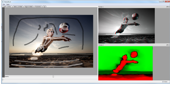
Figure 1: An example of our user interface. Sparse scribbles are drawn on the left, and the resulting stereo is displayed on the right along with a visualization of disparity.
