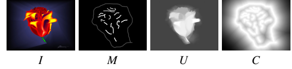
Figure 2: Scribble Propagation. (I) Input image, (M) user provided scribbles, (U) dense scribble propagation, (C) confidence map, the distance transform to nearest scribble.
