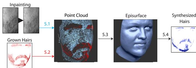
**Figure 13:** Episurface reconstruction overview. The episurface is reconstructed from the inpainted images (blue) where the surface is visible and from the grown hairs (red) where it is covered with hair. From the episurface, additional hairs can be synthesized.
