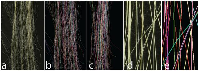
**Figure 22:** Synthetic hair test. Given a sample of long synthetic hair (a), the system reconstructs the 3D hairs shown in (b) and (c). A close-up of the input image and the corresponding reconstructed hairs are shown in (d) and (e). Notice how most fibers are correctly reconstructed.
