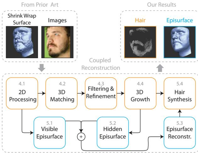
**Figure 3:** Main stages of the algorithm. A preliminary step to the processing is to obtain a first estimate of the 3D model using the method in [Beeler et al. 2010]. The algorithm then explicitly detects and reconstructs hair fibers (top flow) and uses this information to provide a better estimate of the underlying surface (bottom flow). This surface, called the skin episurface, is in return used by the hair reconstruction to synthesize new hairs.
