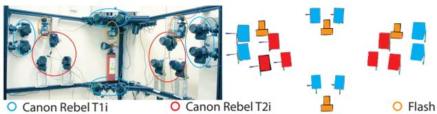
**Figure 17:** Setup used to capture the data. The setup consists of 8 Canon Rebel T1i cameras equipped with 85mm lenses to capture the full face and 6 Canon Rebel T2i cameras equipped with 100mm lenses to capture the chin area. The subject is illuminated with 4 Canon Flashes (430EX, 580EX).
