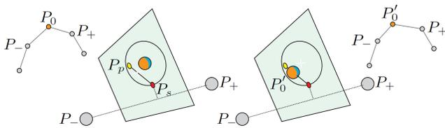
**Figure 9:** The refinement stage. The point  $P_0$  with neighbors  $P_+$  and  $P_-$  is refined on the plane normal to  $P_+ - P_-$ . The refinement computes within a local neighborhood the point  $P_p$  that has highest data fidelity and the point  $P_s$  that has highest smoothness. The refined position  $P'_0$  is computed as the weighted average of these two points as described in Section 4.3(a).
