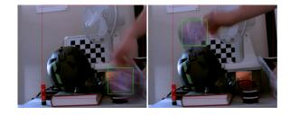
**Figure 7:** Our method accurately tracks the position of the DVD even in the case of very strong motion blur in the video image. The red rectangle shows the overlap region of the two sensors, i.e. the area of the video frame covered by the DVS.
