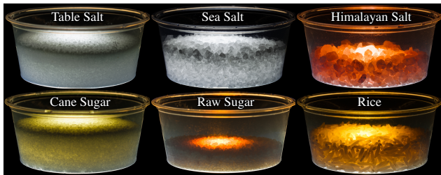
Figure 3: A selection of real granular materials from Figure 2 illuminated from underneath with a cell phone’s flash light to reveal their translucency. Granular materials can exhibit long-range light transport that still retains complex small-scale structure. Each HDR capture was individually tonemapped for display.
