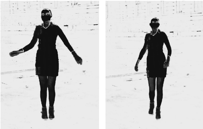
Fig. 2: Raw silhouettes extracted using Gaussian mixture model and graphcut for two random frames from the video. No further post-processing is applied.
