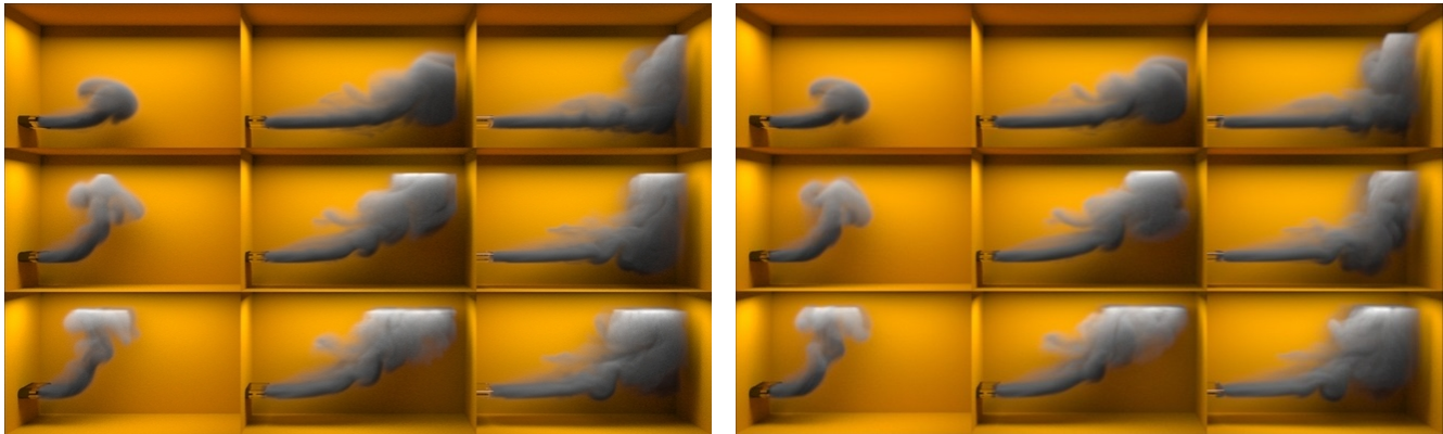
Fig. 2. Ground truth (left) and the CNN-reconstructed results (right) for nine sample simulations with varying buoyancy (rows) and inflow velocity (columns). Despite the strongly varying dynamics of the ground truth simulations, the outputs of our trained model closely reconstruct the reference data.
