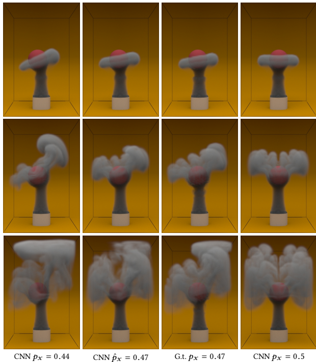
Fig. 8. Interpolated result (second column) given two input simulations (left and right) with different obstacle positions on the x-axis. Our method results in plausible in-betweens compared to ground truth (third column), even in the presence of large discrepancies between the input flow states.
