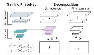
Figure 5: **Hierarchical training.** On the left, PhaseNet takes as input the decompositions  $R_1$  and  $R_2$  of the input frames. In this example the two lowest levels are being trained (m=2). Corresponding blocks are displayed in green. The other blocks (in gray) will be added at the next iteration. On the right, we have the ground truth frame decomposition R. To reconstruct the predicted image, we use ground truth values for the layers not being trained yet.
