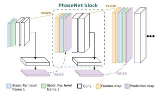
Figure 4: **PhaseNet block.** Each block of the PhaseNet takes as input the decompositions of the input frames at current level (shown in blue and green). Each level performs two successive convolutions with batch normalization and ReLU. From the intermediate features map, each block predicts the response (amplitude and phase) at current level with one convolution layer followed by the hyperbolic tangent function. Feature map and predicted values are reused in the next block after resizing.
