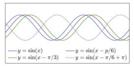
Figure 2: **Interpolation as phase shift.** The translation of a simple sinusoidal function (blue to green) can be expressed by the phase difference. To estimate the middle signal, phase-based interpolation needs to determine the correct phase value among the two possible solutions in purple.
