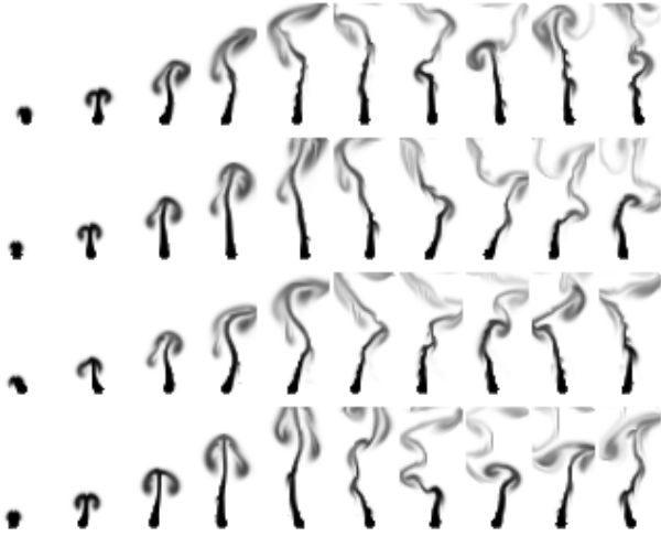
Figure 16: Four example sequences of our moving smoke dataset. For visualization purposes we display frames 20 to 200 with a step size of 20 for the respective scenes. The smoke density is shown as black.
