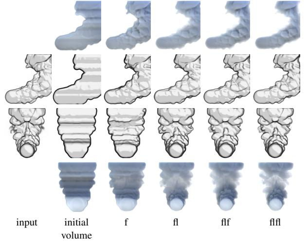
**Figure 4:** From two input sketches depicting the front and left views, we compute the initial volume and then alternately optimize the front (*f*) and left (*l*) view density reconstructions with an updater CNN. The intermediate density fields and corresponding sketches illustrate the convergence.
