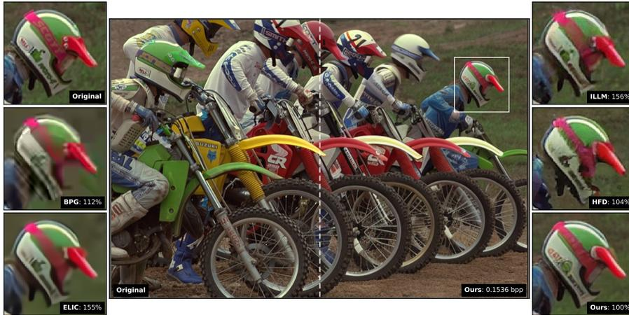
**Fig. 1:** Visual examples of our proposed method and various classes of image compression codecs. Traditional (BPG [1]) and autoencoder-based (ELIC [20]) codecs suffer from blocking or blurring, and reconstructions from GAN-based (ILLM [34]) and previous diffusion-based (HFD [24]) methods contain high-frequency artifacts. Our proposal is as realistic as the original image while recovering a high level of detail. Bitrates are shown relative to our method. Best viewed digitally.
