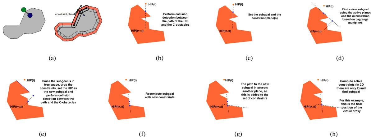
Figure 143: 3DoF haptics: Virtual proxy
