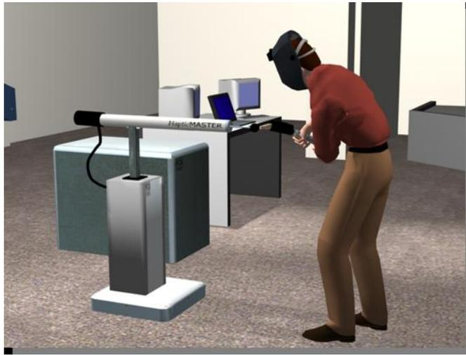
Figure 7: Virtual welding simulator – Image courtesy of FCS Control Systems, The Netherlands
