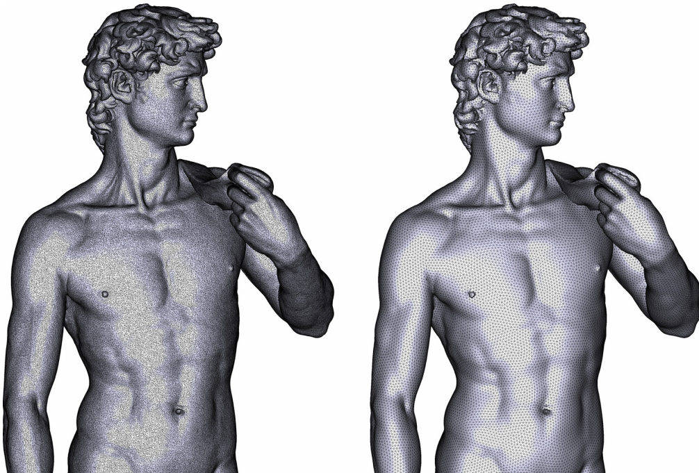
Figure 10.6: Isotropic remeshing using overlapping parameterizations.
