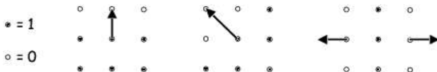
Central difference. Orientation of the gradient in dependence of the scalar field.
