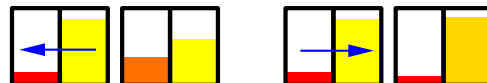
Figure 4: This figure illustrates the donor-acceptor method in which the amount of mass transferred is proportional to the mass of the donor. The voxels on the left show the transfer of mass and energy according to the flow, indicated by the blue arrow. The two voxels on the right represent the scenario with reversed flow of the same magnitude. Density is represented as height, and unit energy is represented as color. Corresponding amounts of energy are sent with the mass.
