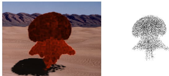
Figure 9: A fireball after one second of simulation time. Tracer particles from the fluid simulation determine the position and coloration of the fireball.
