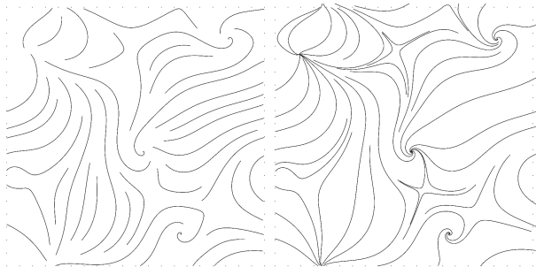
Fig. 3. Left: Euclidean distance metric (window size is zero), Right: Similarity distance metric (window size is six percent of domain width). Both images use 50 streamlines.
