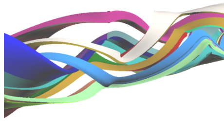
Fig. 8. Visualization of several stream volumes. A stretching, rotating and diverging motion between adjacent volumes can be observed.
