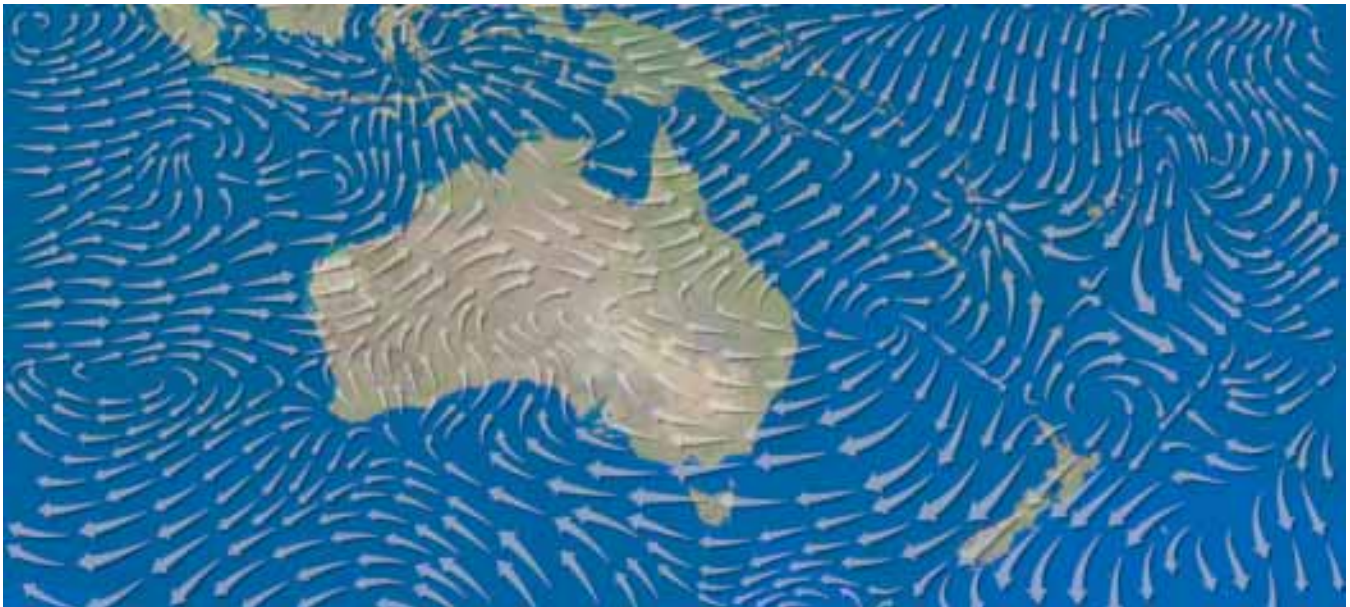
Figure 7: Chains of arrows indicate wind direction and magnitude over Australia. The arrows were deposited along streamlines created by streamline optimization. Higher velocity is indicated by larger arrows. The vector field data was calculated using a numerical weather model.
