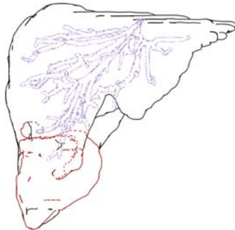
Figure 7: Hidden feature lines are rendered as dashed lines. With this technique additional information concerning a tumor and the intrahepatic vasculature are included in a visualization.
